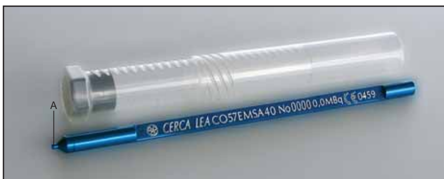
A: radioactive deposit Length: 185 mm
